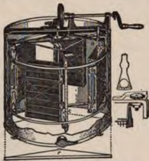
Fig. 322. A modern type of automatic honey-extractor.
